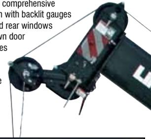
35-58 ft (10.7-17.7 m) two-piece bi-fold lattice attachment with 2°, 15°, 30° and 45° offsets
