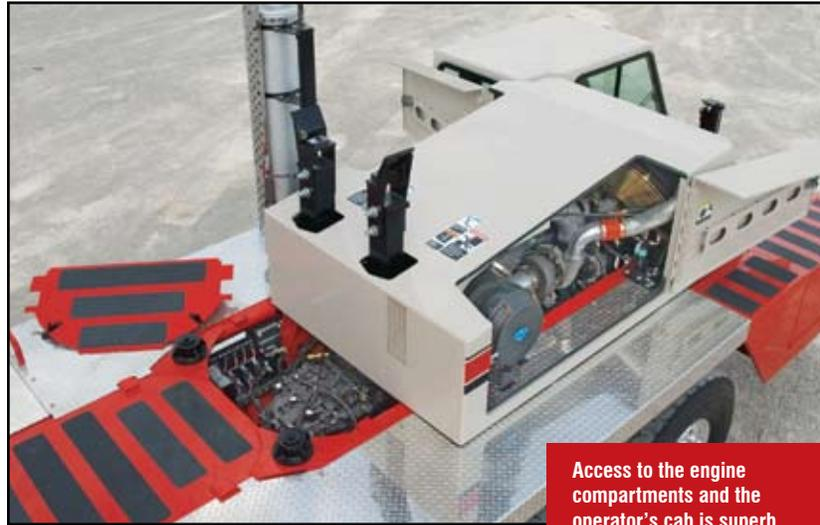
Access to the engine compartments and the operator's cab is superb with strategically-located ladders and steps.
