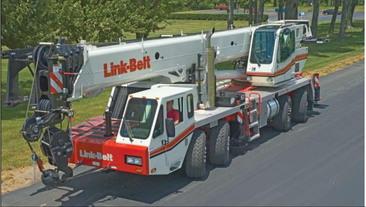
**Steerable all wheel axles, in conjunction with super single tires, makes the HTT even harder to beat on the job-site. And NO changes to the on-outrigger capacity charts.**
